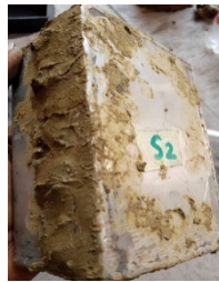
Figure 3.2: Carburization box sealed with clay and sodium silicate
