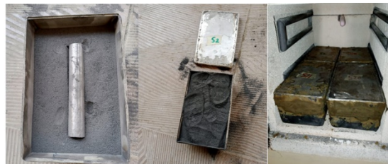
Figure 3.3: Mild steel rod in carburization materials arranged in the furnace
