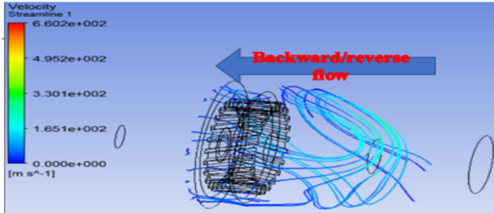
Figure 17: Flow reversal and turbulence flow in the turbine with 10% degradation.
