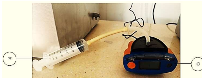
Figure 2. Setup for gas analysis using the Crowcon Analyser
