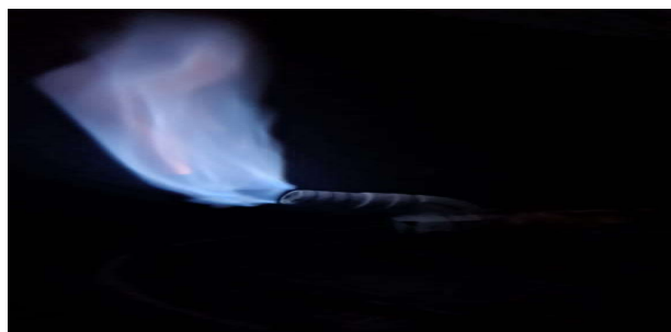
Plate II: Combustion of biogas from PCCDBC
