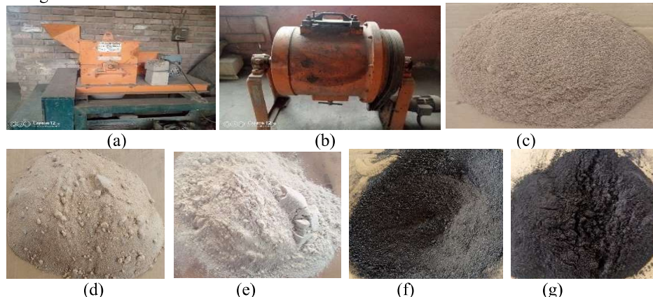
Fig 3: The various machines used and processed raw materials (a) Hammer Mill (b) Ball Milling Machine (c) Rice Husk (d) Processed Gum Arabic (e) Steel Slags (f) Graphite (g) Quartz.
