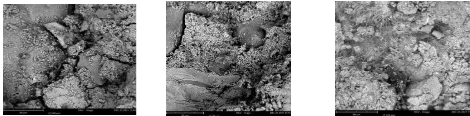
Figure 5: SEM Result for (a) CRD @ 28 days (b) LP at 28 days (c) CKD at 28 days
