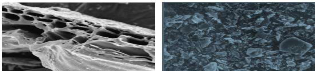
Figure 2: Scanning Electron Microscopy analysis of Greek and Pakistan Rice Husk Ash (RHA)
