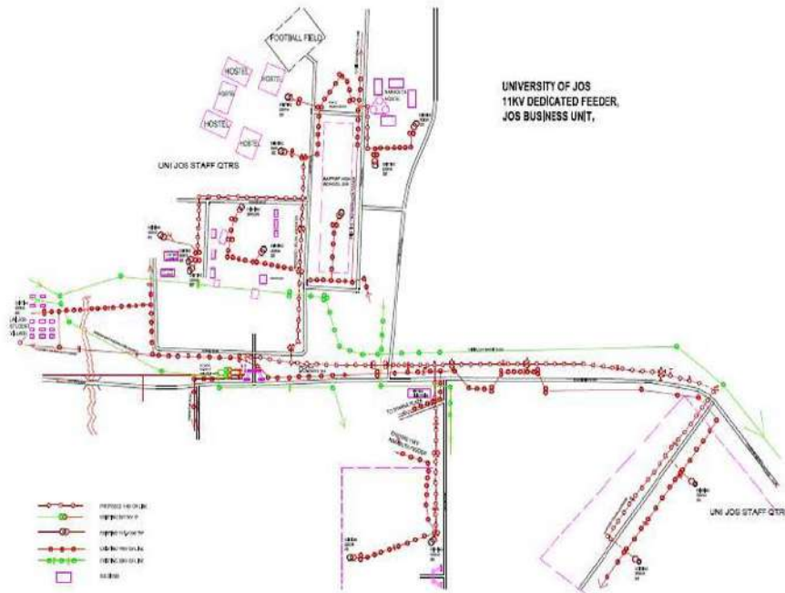
Figure 1. A sketch of the 11 Kv dedicated Feeder of the University of Jos.
