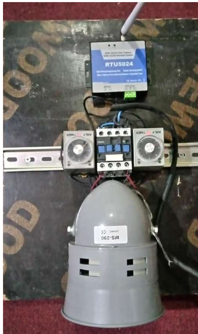
Figure 5: A GSM manned alarm system
