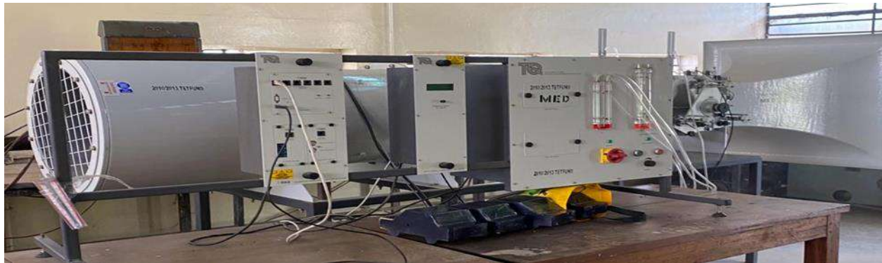
Plate III: A TQ AF100 Subsonic Wind Tunnel used for the determination of sediment flux.
