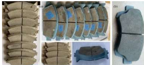
Figure 2: Brake pad (a) Agro composite brake pad (b) Asbestos lined brake pad
