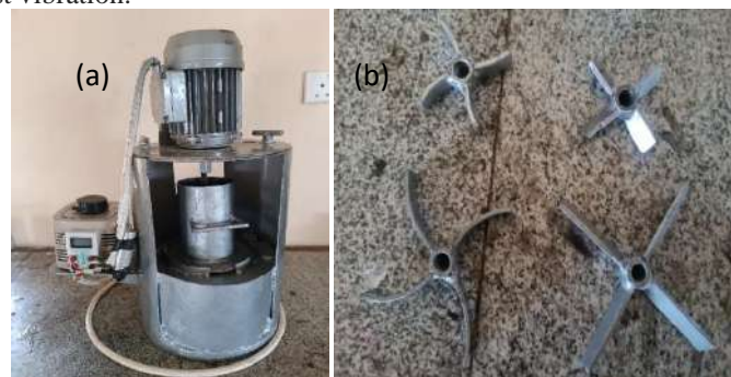
Figure 3: (a) fabricated mixer (b) fabricated impellers
