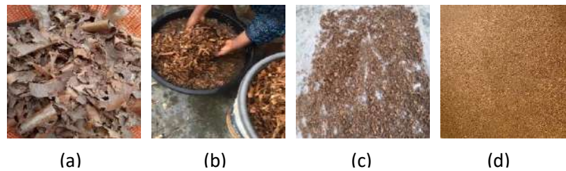
Figure 1: Preparation of cassava periderm powder from (a) cassava periderm, (b) washing of the periderm, (c) sun drying, and, pulverised to obtain (d) cassava periderm powder.
