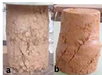
Fig. 9 Failure plane for 14-day curing a) shearing axially deformation b) bulging shape
