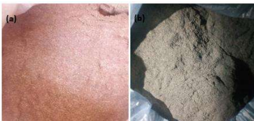
Figure 1: (a) Milled coconut shells (b) Carbonized coconut shell particles.
