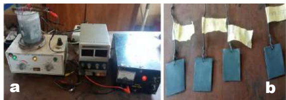
Figure 1: Photograph of the electrodeposition process showing (a) equipment and (b) coated samples
