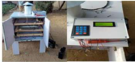
Figure 9: Designed Solar-based Dryer (Prototype)
